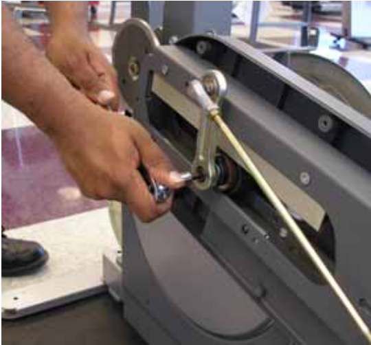
Fig. 5: removing the crank extension bolt
